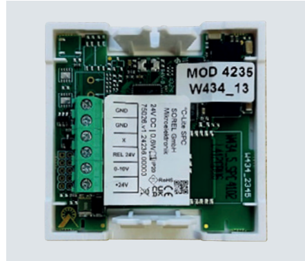
Figure 2. Underside of controller showing terminal blocks
