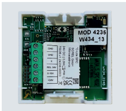
Figure 2. Underside of controller showing terminal blocks
