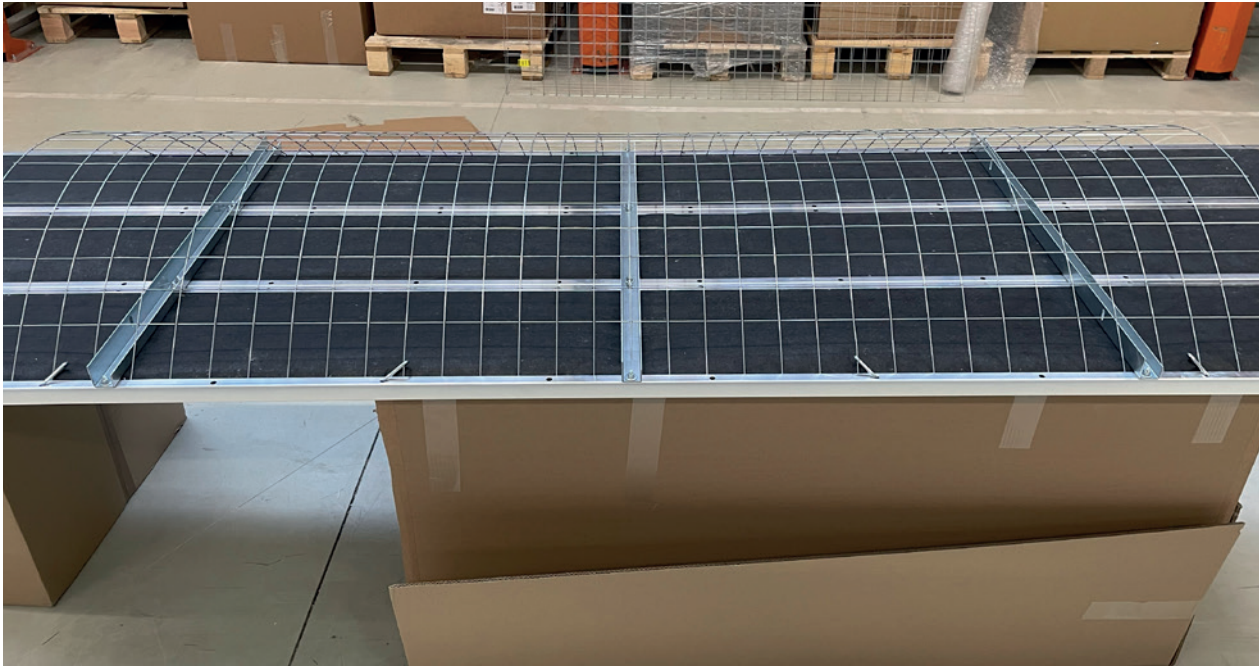
Figure 5. Array of carabiner clips holding mesh to side flanges
