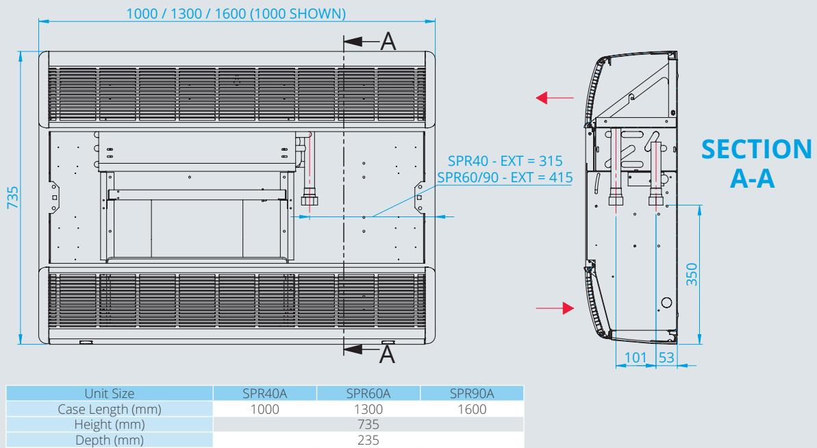
Units shown with rh connections dimensions same with lh connections. Connections through knock-outs in bottom panel or through plinth. Plinth not shown
