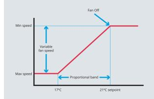
The chart shows how the controller varies the speed of the fan in response to the difference between the actual temperature and the setpoint temperature. Within the proportional band the fan speed is continuously varied to precisely match heat output to the required load.
