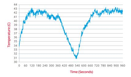
The chart shows temperatures measured on the outlet grille of an SPC fan convector utilising 'Active LST' control. The outlet grille and top panel are the hottest points on the casing.
