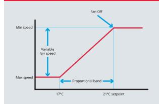
The chart shows how the controller varies the speed of the fan in response to the difference between the actual temperature and the setpoint temperature. Within the proportional band the fan speed is continuously varied to precisely match heat output to the required load.
