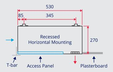
Suitable for T-bar or Plasterboard, air drawn from the ceiling void
