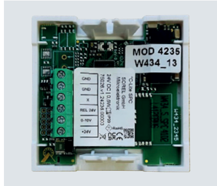
Figure 2. Underside of controller showing terminal blocks
