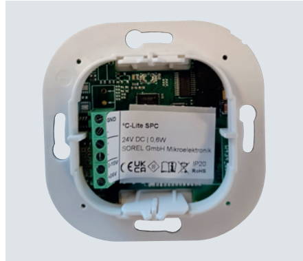
Figure 2. Underside of controller showing terminal blocks
