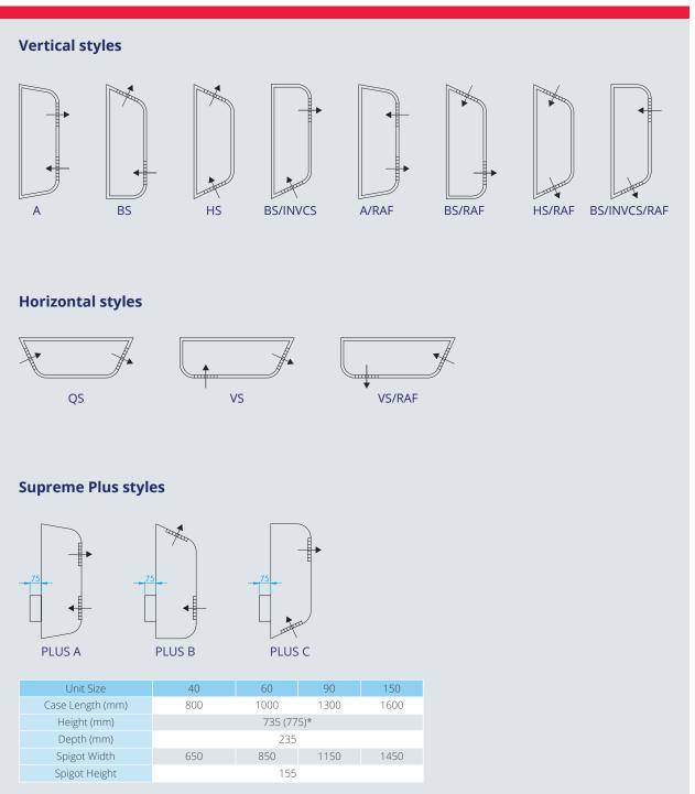
\*Plus unit has increased height Extended casing is not available on plus unit Pipe connections ¾" BSP on all models (½" on lowflow heat exchangers)
