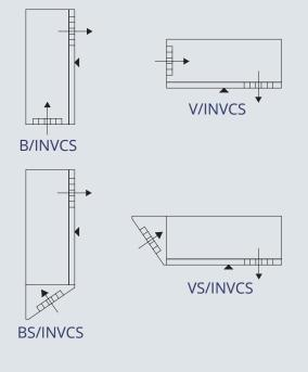
Inverted case + reversed air flow styles
