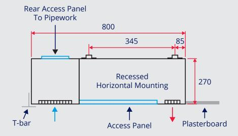
Suitable for T-bar or Plasterboard, air drawn from room below.
