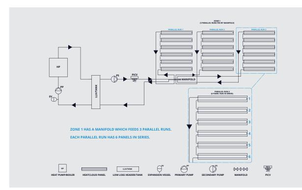
Figure 8. Multi-zone piping example
