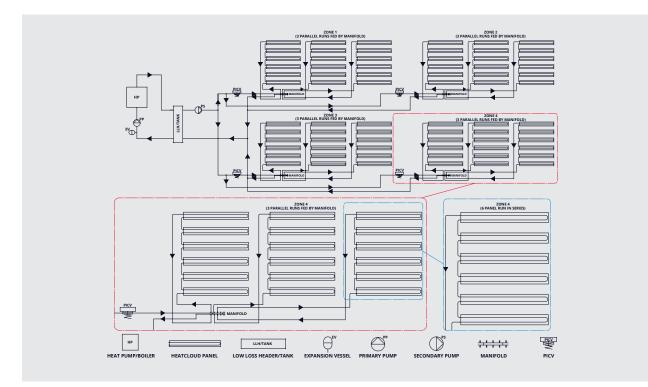
Figure 7. Example of single zone piping
