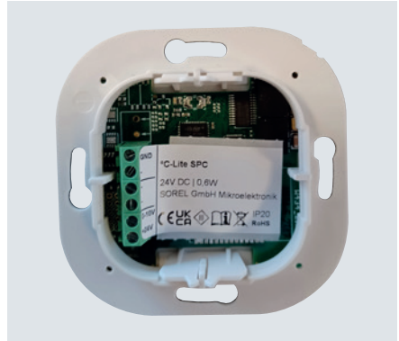
Figure 2. Underside of controller showing terminal blocks
