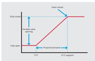
The chart shows how the controller varies the valve opening in response to the difference between setpoint and actual temperature. Within the proportional band the valve opening is continuously varied to allow the heater to match the required load.
