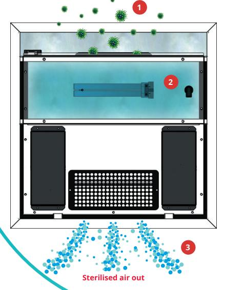
**Contaminated air** is drawn into the unit by the fan
