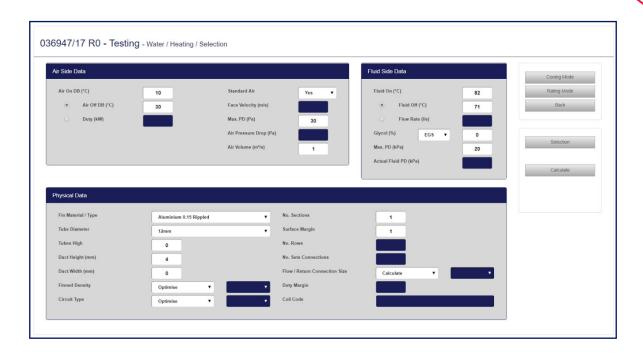
While entering your coil specifics, the SPC Online Coil Selector Software will test your inputs against a list of requirements and validation. Any issues with your coil selection that are either not possible or advised against will be highlighted in red. A short explanation will appear at the bottom of the selection to guide you through the selection. For example:
