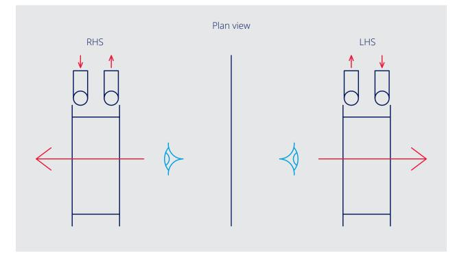
For water coils it is conventional to make the flow connection at the bottom of the coil and the return connection at the top. This assists in ensuring that air is easily vented from the upper connection and that the coil can be drained of water via the lower connection. It is acceptable to reverse this to suit the airflow direction if it has been wrongly specified.
